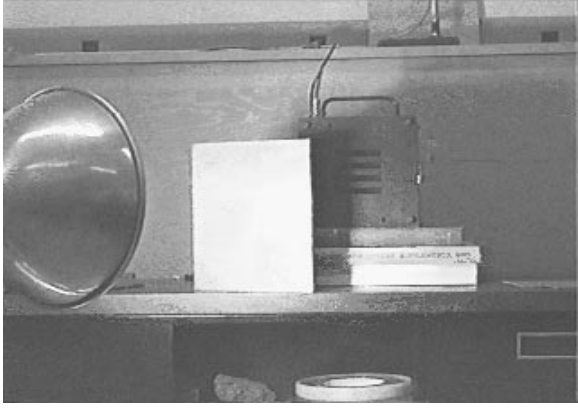
Figure 5: Visible image of the scene used for the demonstration. The reflective plate and differential source are illuminated by an incandescent lamp. Here the lamp intensity is much greater than when the experiment was performed so that the reflected light can be seen.
