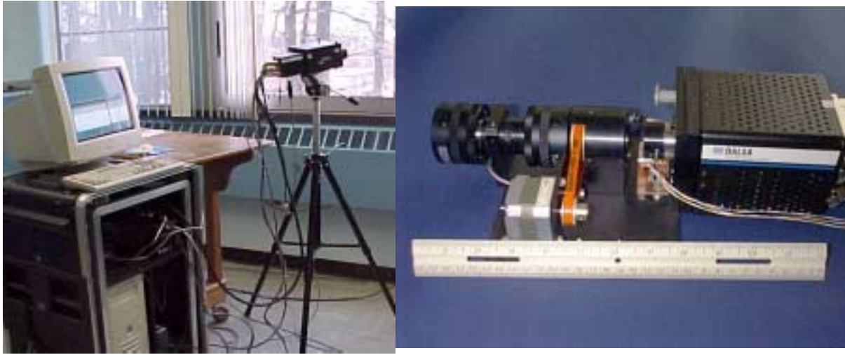
Figure 3: Photos of the Visible/NIR CTHIS instrument and supporting computer system on the left. A close-up of the sensor optics assembly and camera head is shown on the right.
